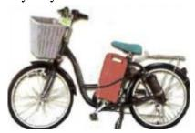
Type approved two-wheeled vehicle which is powered mainly by human exercise and assisted with electricity, with a maximum speed of 25 km/h, and weighs less than 40 kg.
